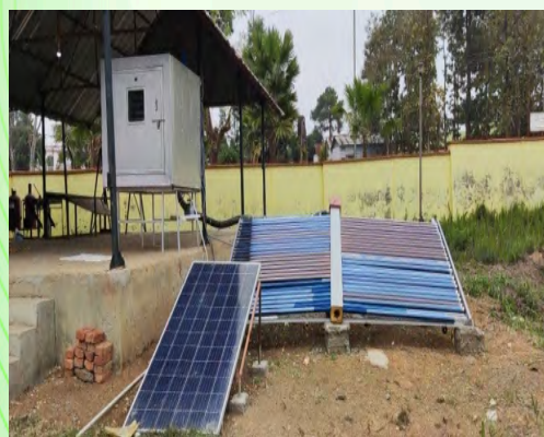
Fig 62. Solar dryer system cum heat spacing as per NISE specification for 180 kg capacity of fruits & vegetables
